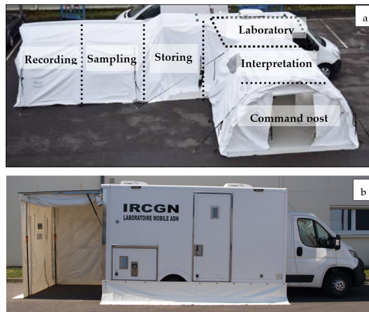
Figure 4. (a) The first mobile DNA Laboratory is made of a Renault Master L3H2 fitted for DNA analysis. It allows transport of all the equipment in the field. Once deployed, different areas are dedicated to an analytical step, limiting the risk of DNA contamination. (b) The mobile DNA laboratory version 2 is a container sealed on a van which is more compact and does not need side tents to be deployed.
