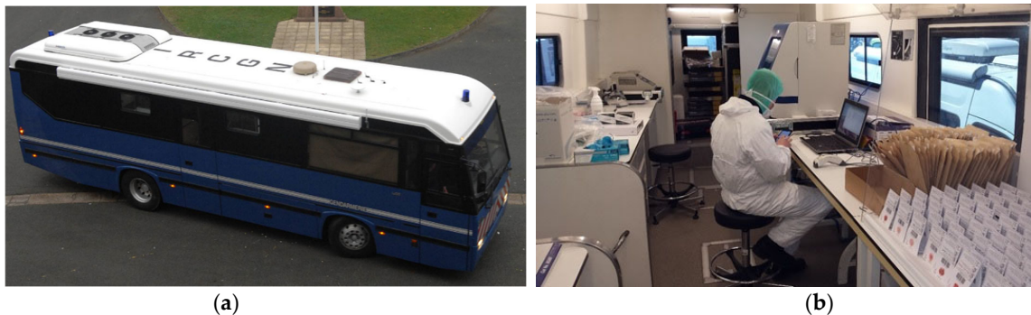
Figure 3. (a) French Gendarmerie Forensic Laboratory bus (b) fitted for DNA analysis with dedicated areas for drying and sampling FTA ® cards (foreground) and (b) for performing analyses (background).
